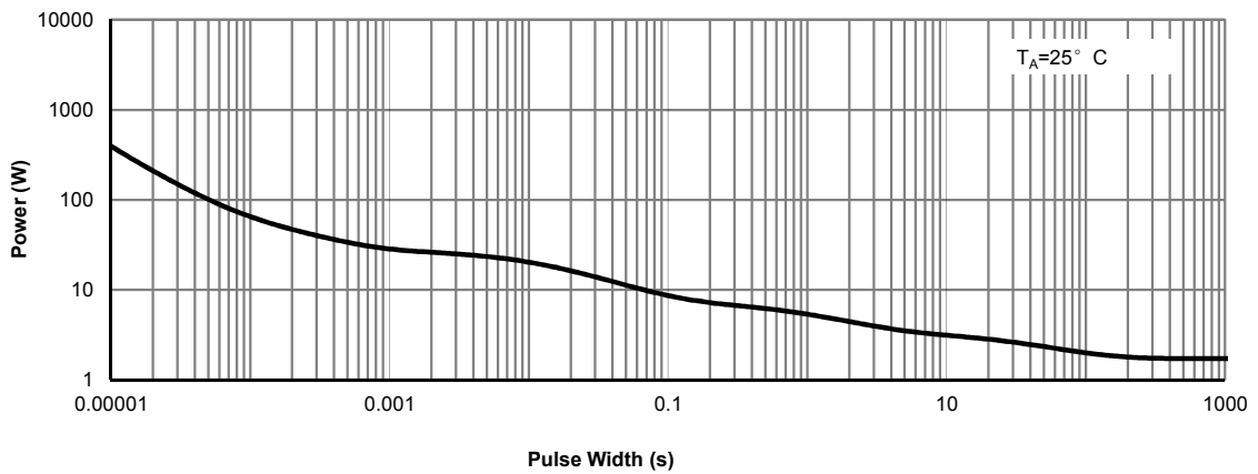
Figure 14: Single Pulse Power Rating Junction-to-Ambient (Note H)
