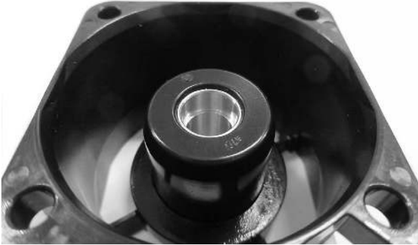
Fig. 3 Coating of electrical live parts (New 28 mm thick model)
