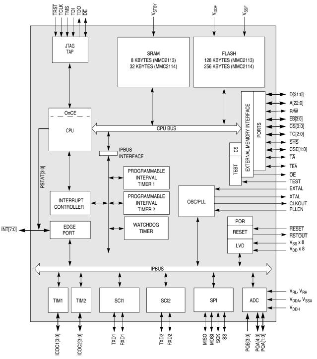
Figure 1. MMC2114 Block Diagram
