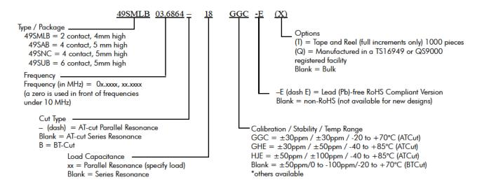
Part Number Examples: Freq 5.1234MHz,  $\pm 30$ ppm calib,  $\pm 30$ ppm stability, -20 to +70°C, 16pF = 49SMLB05.1234-16GGC
