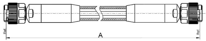
All dimensions are in mm; tolerances: ± 3mm for A ≤ 300 mm; ± 1% for A > 300 mm
