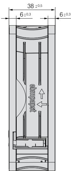
Rotor protrusion max. 0.6 mm.
