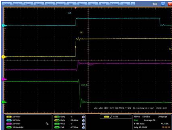
Figure 16: Turn ON output current characteristics (1)
