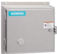
Non-reversing contactor, Size 1 3/4, Three phase full voltage, Contactor amp rating 40A, 3 wire (NO aux included), 240V 50Hz / 277V 60Hz coil, Non-combination type, Encl NEMA type 4X 304 S-Steel, Water/dust tight noncorrosive, Extra-wide enclosure
