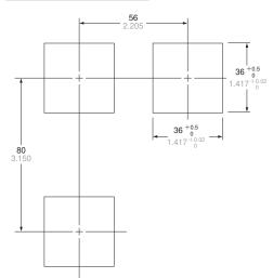
Note: The panel thickness should be 1 to 3.2 mm 0.039 to 0126 in.
