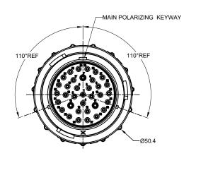
1. MATERIAL: HOUSING: THERMOPLASTIC; BLACK SEAL: SILICONE RUBBER
