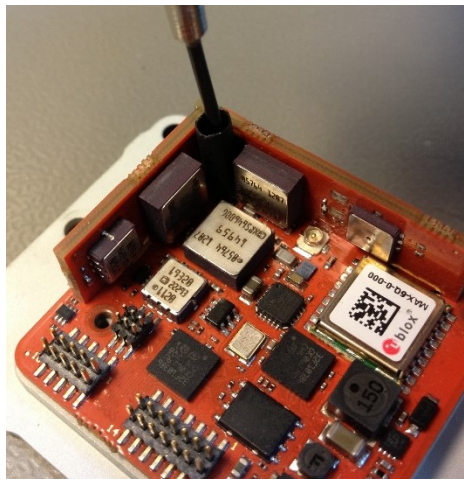
Figure 15: Using a heat shrink tube to position the mounting screws
