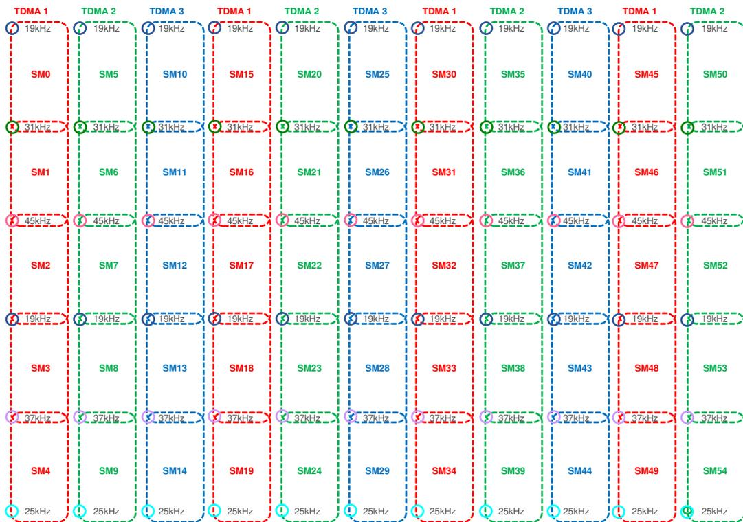
Moreover, the map consists of  $6 \times 11 = 66$  stationary beacons, i.e. 11 beacons of each of the frequencies combined into submaps: 19-31kHz, 31-45kHz, 45-19kHz, 19-37kHz, 37-25kHz.
