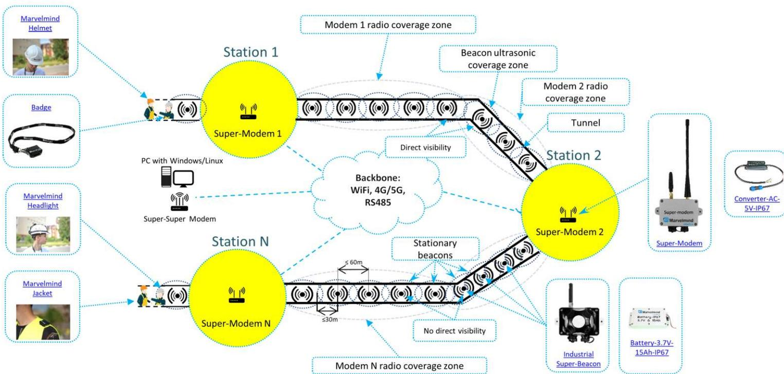
Setup of a Multi-Modem architecture is simple:
