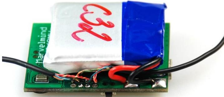
Figure 4: Two external microphones soldering
