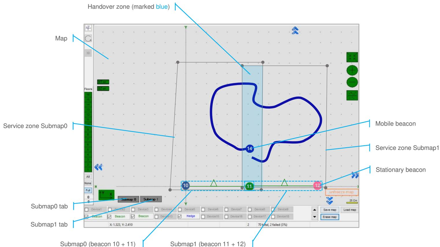
The main parameters of a submap are its **size**, **frequencies** and **TDMA (Time Division Multiple Access) position** of stationary beacons, by which mobile beacons can not only be positioned, but also determine in which submap the mobile beacon is located.
