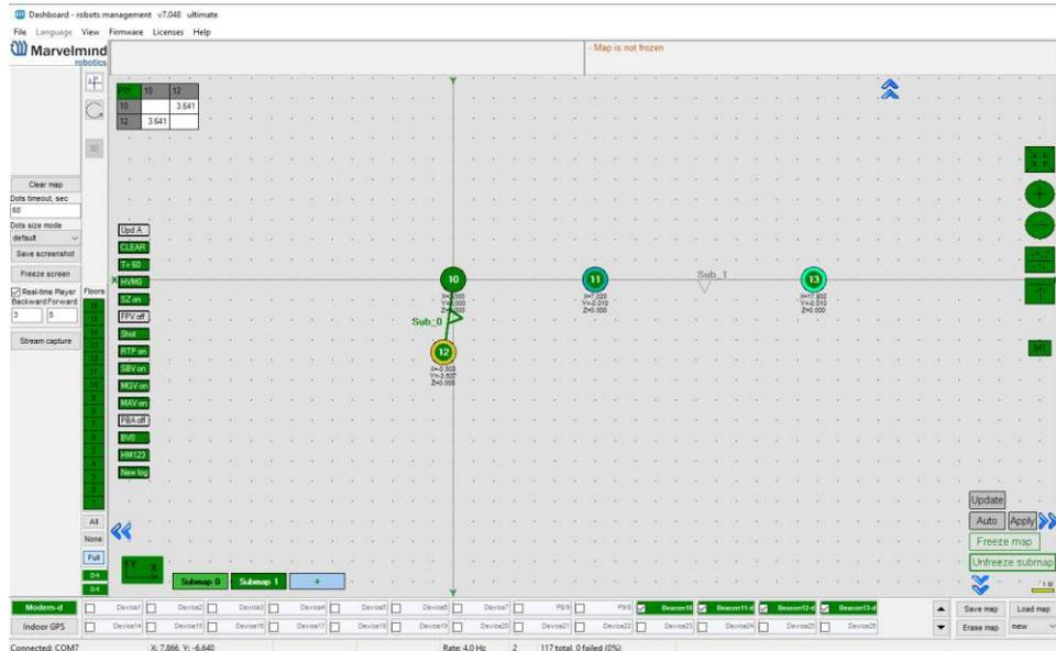
9.16.1.13. After some movement, rotation, and mirroring of submaps, we can locate the submaps close to their real relative location
