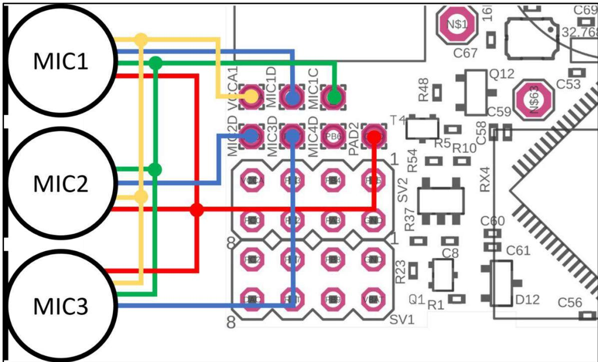
Figure 8: Two External Microphone connection
