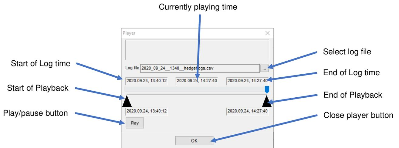
Limited area - distance between black triangles under slider. You can move triangles and zoom, place cursor on the slider + mouse wheel. Triangles limit the area in which player works and the statistics is calculated
