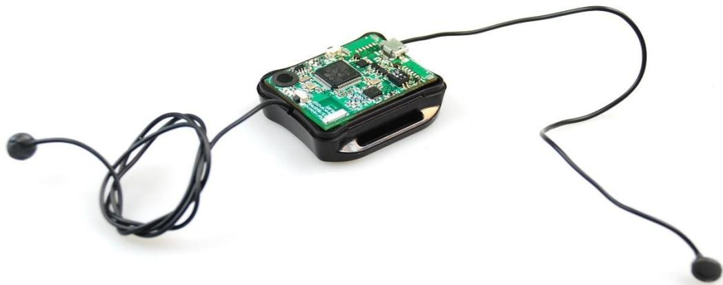
Figure 2: Two external microphones with housing
