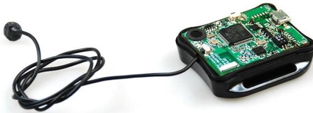
Figure 1: One external microphone with housing
