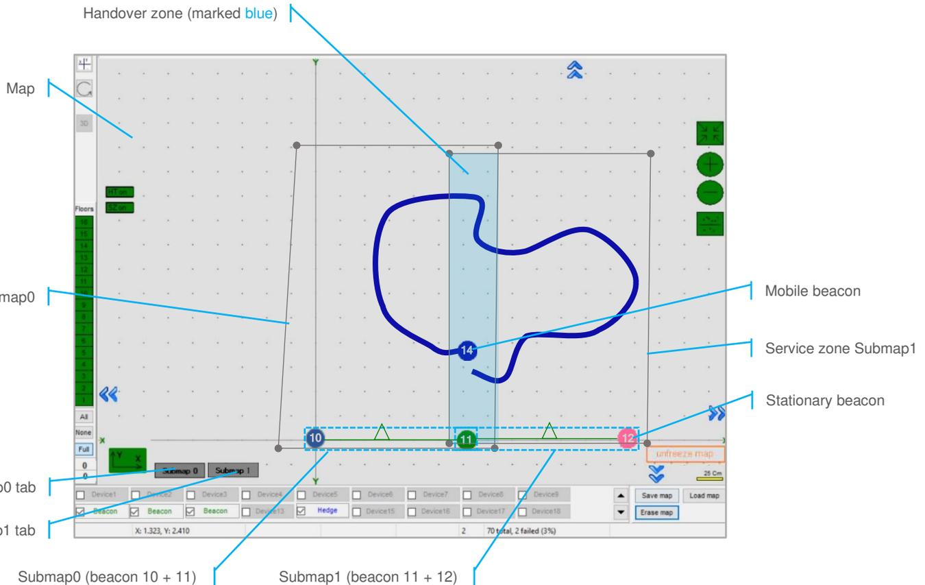
The main parameters of a submap are its **size**, **frequencies** and **TDMA position** of stationary beacons, by which mobile beacons can not only be positioned, but also determine in which submap the mobile beacon is located.
