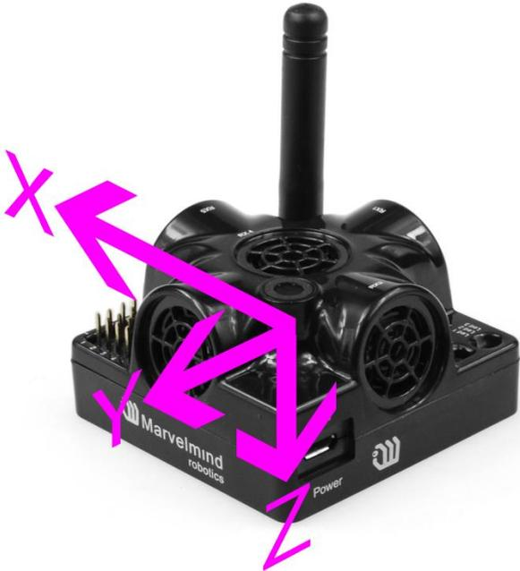
HW v4.9 IMU axis positions
