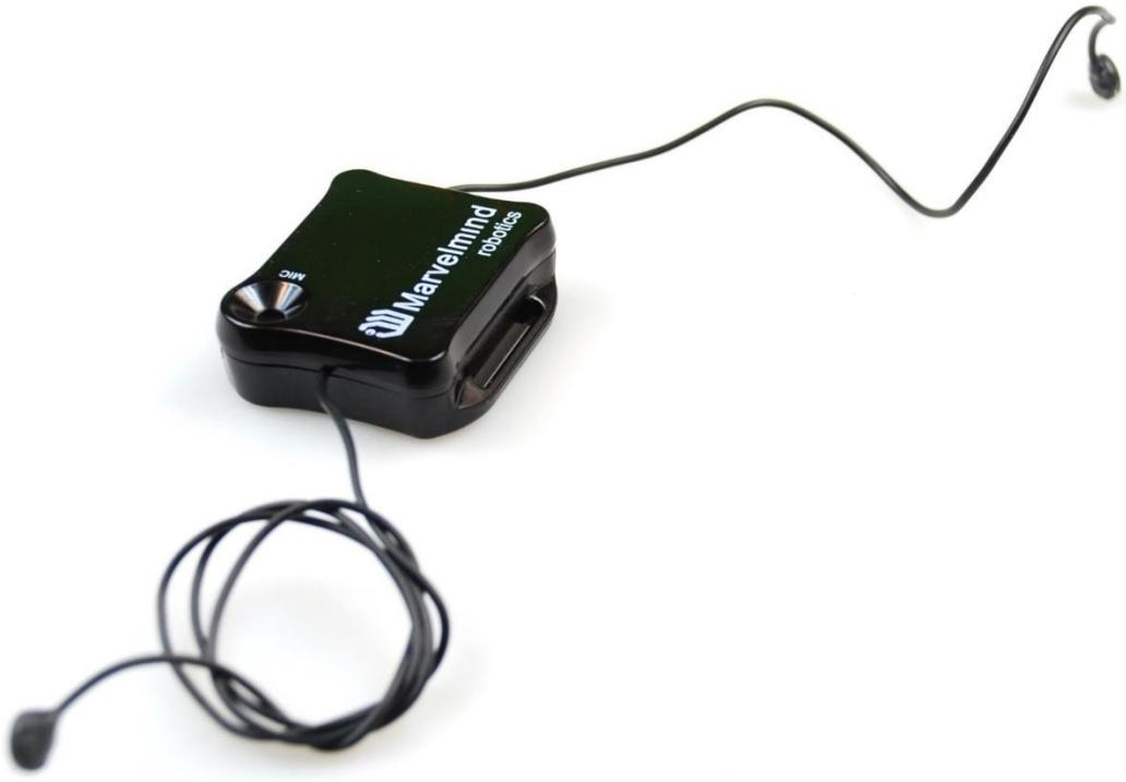
Figure 7: Two External Microphones final view
