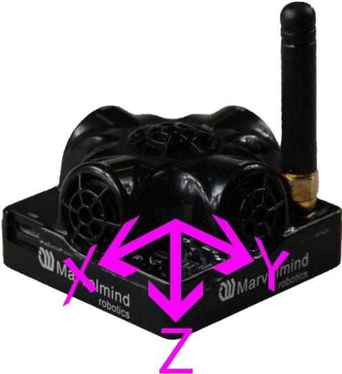
Mini-TX IMU axis positions
