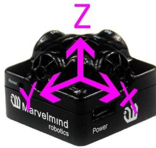
Mini-RX beacon IMU axis positions
