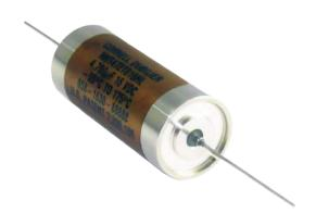
Type HHT has long life and rugged construction for high temperature environments. HHT capacitors are rated for full operating voltage at 175 °C and tested to 2000 hrs at rated voltage and temperature. 5000 hours of life at 150 °C with ripple current ratings up to 10 Arms. ■
