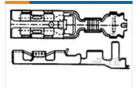
TE Part #353250-2 110 PL EX REC. 20-16AWG PTPHBZ
