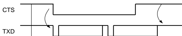
Figure 31-19. Transmitter Behavior when Operating with Hardware Handshaking
