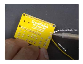
Unfurl and solder the antenna wire on the antenna header hole on the FM board.
