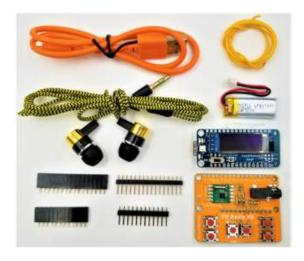
Unwrap the ball and lay out the various kit components. The provided USB cable will be used to program the Azul and can also be used to charge the Lithium Polymer battery. The Azul has the battery charging circuitry built in.
