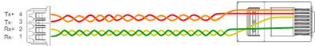
Figure 9: Ethernet cable pinout
