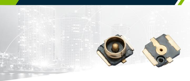
Part of the Taoglas SMD Mount Receptacle the RECE.20369.001E.01 is a 3-pad type wire-to-board SMD Receptacle solution that is ultra-small, lightweight and low profile (1.6mm MAX.) with an operational frequency range of DC to 6 GHz. Taoglas the RECE.20369.001E.01 is gold plated to have superior performance and allow easy mounting of the male RF connector.
