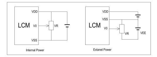
$V_{\text{DD-}}V_0$ : LCD Driving voltage VR: 10k~20k
