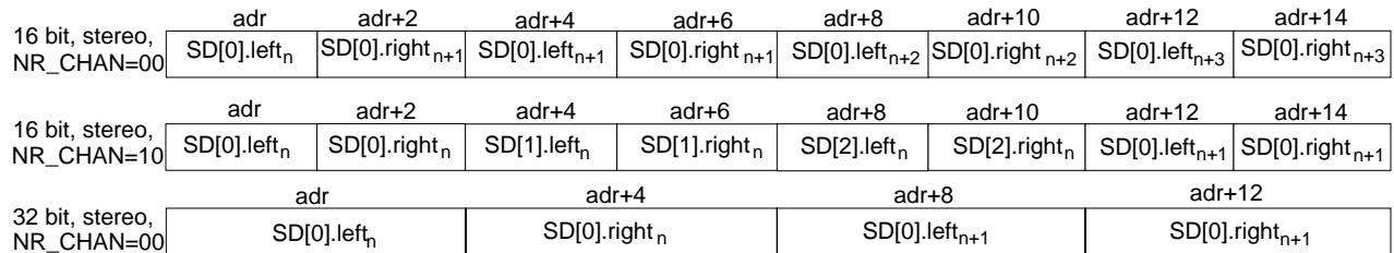
Figure 2: Examples of Audio Out Memory DMA Formats
