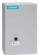
Non-reversing contactor, Size 3 1/2, Three phase full voltage, Contactor amp rating 115A, 3 wire (NO aux included), 240V 50Hz / 277V 60Hz coil, Non-combination type, Enclosure NEMA type 1, Indoor general purpose use, Standard width enclosure
