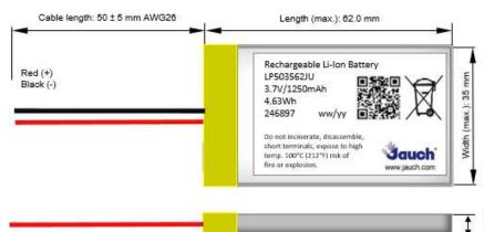
Thickness (max.): 5.0 mm (deliver status) 5.4 mm (after cycling)
