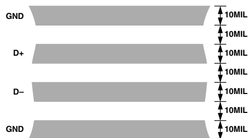
Figure 5. Arrangement of Signal Tracks
