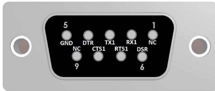
Figure 6. DB9 Pinout
