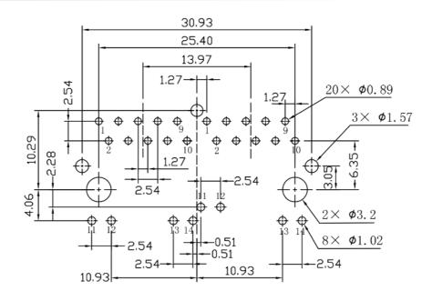
Suggested PCB Layout (Top View) Dimensions are in millimeters with the following tolerances:  $X.XX = \pm 0.10$
