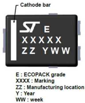
Figure 10. PSMC (TO-277A) marking
