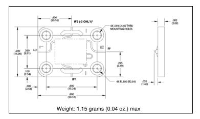
\*For the base model, only IF1 port is connected. For the "-2" model only, the IF2 port is connected.
