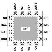
\*THERMAL PAD MUST BE CONNECTED TO NEGATIVE SUPPLY:  $V_{S}\text{-}.$  QFN PACKAGE CAN BE USED IN DUAL SUPPLY APPLICATIONS.
