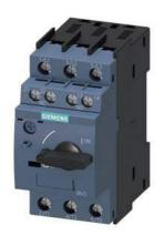
Circuit breaker size S00 for transformer protection A-release 3.5...5 A N-release 104 A screw terminal Standard switching capacity with transverse auxiliary switches 1 NO+1 NC
