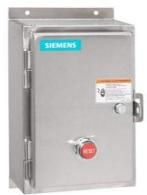
Non-reversing motor starter Size 1 3/4 Three phase full voltage Solid-state overload relay OLRelay amp range 10-40a 220-240/440-480VAC 60HZ coil Combination type Water/dust tight non-corrosive
