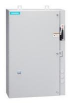
Non-reversing motor starter Size 1 Three phase full voltage Solid-state overload relay OLRelay amp range 0.25-1A 24Vdc coil Combination type 30Amp non-fusible disconnect Enclosure NEMA type 4/12 Water/dust tight weather proof Extra-wide enclosure
