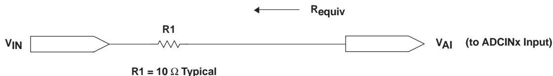
Figure 41. Typical ADC Input Pin Circuit
