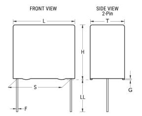
**General Information** Series PFR/F411 Dielectric Film/Foil Polypropylene Style Radial Features Pulse RoHS Yes Lead Wire Leads AEC-Q200 No Component 0.391 g Weight An Operating Temperature Up To +105C Is Allowed Under Certain Conditions. Please Consult Miscellaneous KEMET For Details.
