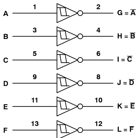
$V_{DD} = \text{Pin}14$
