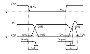
Note 2: Switching loss measurement waveforms
