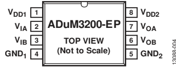
Figure 4. ADuM3200-EP Pin Configuration
