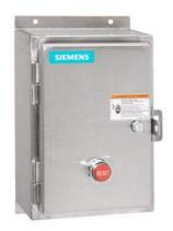
Non-reversing motor starter Size 1 Three phase full voltage Solid-state overload relay OLRelay amp range 0.25-1A 550/575-600 50/60HZ coil Combination type Water/dust tight non-corrosive
