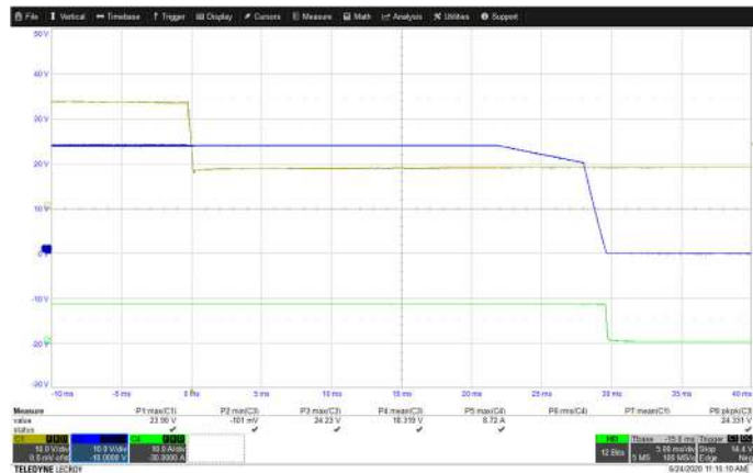
Hold Up/Interruption Time: Measured hold up time with 24Vo/200W Ch1: Vin Ch3: Vout Ch4: Iout (NOTE: for models with Hold Up option)
