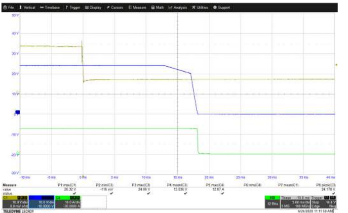
Hold Up/Interruption Time: Measured hold up time with 24Vo/300W Ch1: Vin Ch3: Vout Ch4: Iout (NOTE: for models with Hold Up option)
