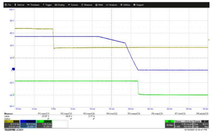
Hold Up/Interruption Time: Measured hold up time with 54Vo/300W Ch1: Vin Ch3: Vout Ch4: Iout (NOTE: for models with Hold Up option)
