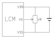
V<sub>DD-</sub>V<sub>0</sub>: LCD Driving voltage VR: 10k~20k
