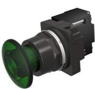
30mm BlackMax, Epoxy Coated Corrosion Resistant Complete Metal Unit Illuminated Push-Pull Operator Full Voltage, 24V AC/DC LED Lamp Mushroom Head Cap Small 1 3/4" (44.5 mm) Plastic, Green 3 Position Momentary UL Listed, CSA Certified NEMA 1,3,3R,4,4X,12,13 & Automotive Standards
