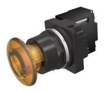
30mm BlackMax, Epoxy Coated Corrosion Resistant Complete Metal Unit Illuminated Push-Pull Operator Transformer type, 600V AC LED Lamp Mushroom Head Cap Small 1 3/4" (44.5 mm) Plastic, Amber 3 Position Momentary UL Listed, CSA Certified NEMA 1,3,3R,4,4X,12,13 & Automotive Standards
