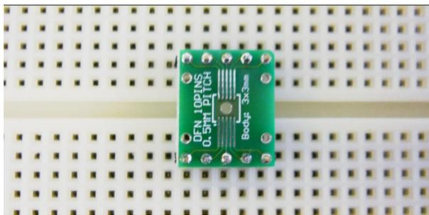
This product is an DFN to DIP adapter with a twist. These have our patented "ez" technology which means that soldering the surface mount component is simple, and as with all of our "ez" boards, we are the only company with a patented solution for easily soldering surface mount parts. Included in the package are two .5mm pitch adapter boards for 10 leads and a row of headers to use the boards with a breadboard.
