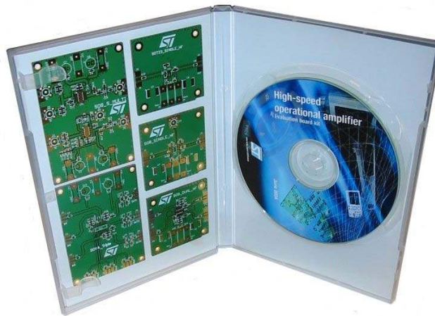
Figure 44. Evaluation kit for high-speed op-amps
