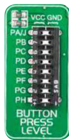
Figure 6-5: Button press level DIP switches (tri-state)
