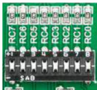
Figure 6-2: Tri-state DIP switch on PORTC
