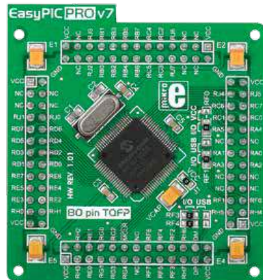
2 Figure 4-6: Standard 80-pin MCU card with PIC18F8520 .
