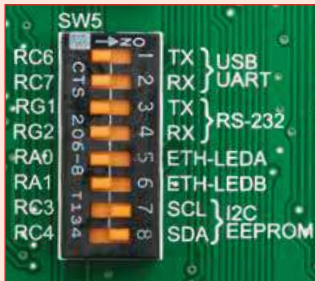
Figure 19-1: Activate SW5.7 and SW5.8 switches to enable pull-up resistors in I 2 C lines of Serial EEPROM.
