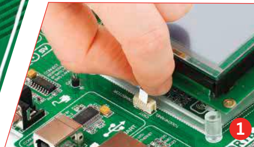
Figure 14-1: Put Touch Panel flat cable in the connector
