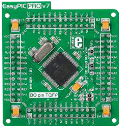
1 Figure 4-5: Standard 80-pin MCU card with PIC18F87J50 , which supports USB.
