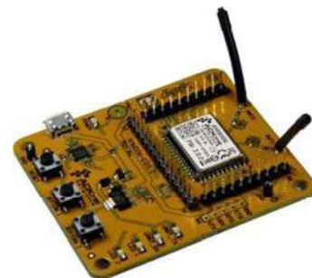
Figure 9 - AMW006-E03 eval board with wire antennas
