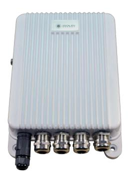
The PoE-3-120, manufactured by Solis Energy, is an unmanaged, hardened, industrial-grade switch designed to reliably connect PoE devices in harsh environments. The PoE-3-120 features three 802.3af/at Gigabit PoE ports and one Gigabit LAN uplink which allow it to handle cutting-edge high-power and high-bandwidth devices.
