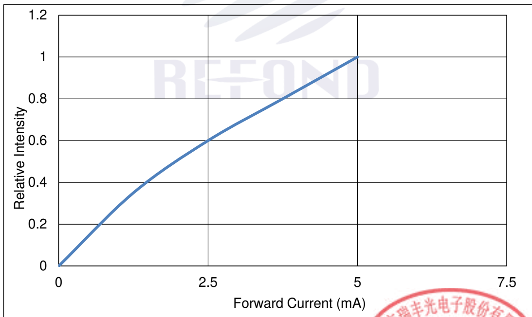
Fig 1-7 Forward Current Vs. Relative Intensity 正向电流与相对光强特性曲线
