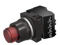
30mm BlackMax, Epoxy Coated Corrosion Resistant Complete Metal Unit PTT / Illuminated Pushbutton Full Voltage, 24V AC/DC LED Lamp Extended Button Plastic Lens, Red 2 Position Momentary with 1 N.O. - 1 N.C. Heavy Duty Contacts, A600/P600 UL Listed, CSA Certified NEMA 1,3,3R,4,4X,12,13 & Automotive Standards
