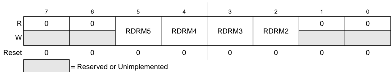
Figure 4-19. Port M Reduced Drive Register (RDRM)
