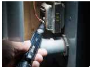
High sensitivity mode for low voltage systems like doorbell transformers
